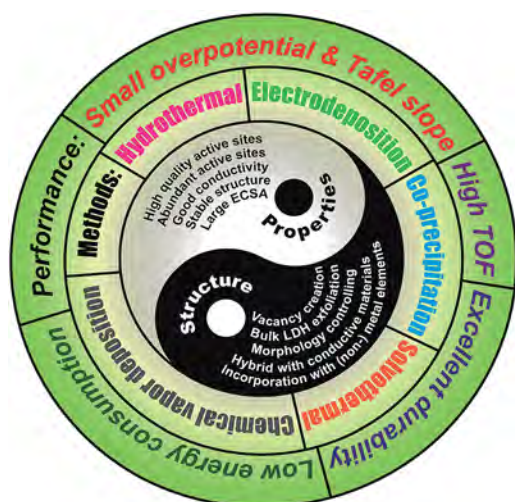
Fig. 5 Schematic representation of typical synthetic methods and development strategies of LDH OER electrocatalysts.
